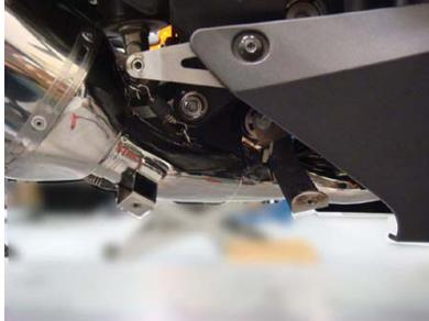
8. **Reinstall lower fairing and exhaust control valve servo cover.**
